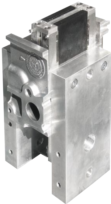
▲ The basis of the valve test bench is a part of a production cylinder head. The gas forces effective on the valve are simulated by air pressure.
